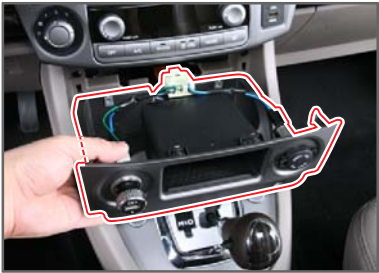
20.Disconnect the power outlet and cigarette lighter connector(A) and remove the center fascia cup holder.
