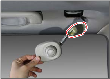
21.Undo the front headlining mounting fasteners (2 off for front and 5 off for rear).
