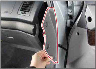
16.Undo the 3 mounting screw rivets on the RH crash cowl side cover and remove the crash cowl side cover.
